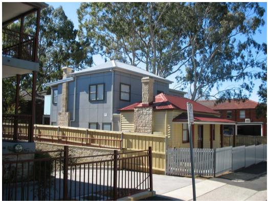
The construction of the new rear section of the house did not comply with the approved plans. Complaints to the Certifier resulted in the new roof being removed and rebuilt with higher walls, as can be seen in the unusually awkward distance between the top of the first floor windows and the eaves.
