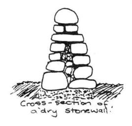
The more usual walls are of shaped stone not requiring a batter and therefore occupying less land, with the stones mortar jointed. Few dry walls remain. Such walls are built with irregular stones and with such skill that no clay or mortar is used. A magnificent example of a wall of this type was located on part of the Victoria Road frontage of the Gladesville Hospital. It was demolished when the road was widened some years ago before such a feature was appreciated.
